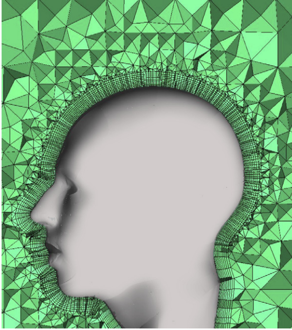
Fig. 2. Refined meshes around the manikin model.
