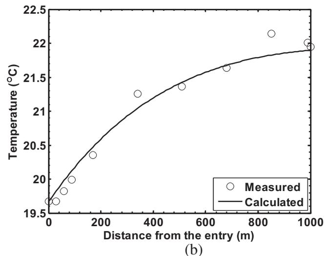
Fig. 9. Comparison of air temperature along the tunnel (a) comparison at 14:00 in Aug the 30th (b) comparison at 4:00 in Sep the 1st.
