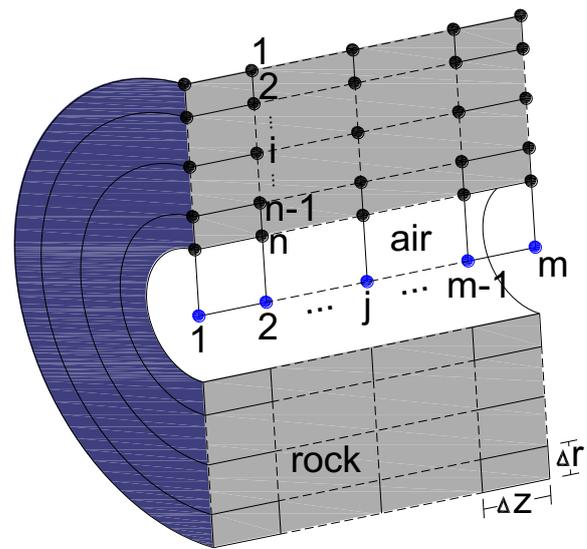
Fig. 4. Discretization of the physical tunnel domain into a numerical mesh.
