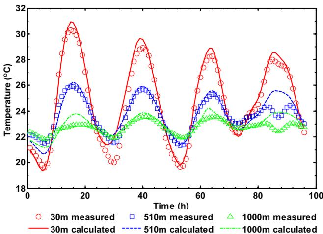
Fig. 8. Comparison of air temperature at different cross sections at  $z = 30$  ( $z/L = 0.027$ ),  $z = 510$  m ( $z/L = 0.46$ ) and  $z = 1000$  m ( $z/L = 0.91$ ).
