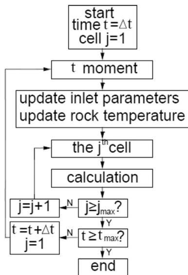
Fig. 5. Computation procedure. The spatial discretization are  $\Delta r = 0.05$  m,  $\Delta z = 10$  m with time steps of  $\Delta t = 300$  s.
