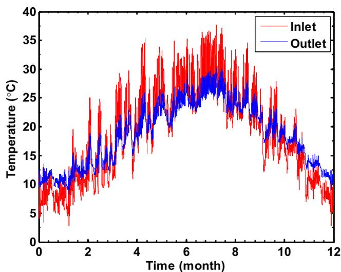
Fig. 11. Inlet and outlet hourly air temperature at the 10th year.
