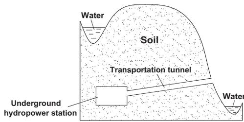
Fig. 1. Schematic of a deeply buried underground tunnel used at underground Hydropower Stations, China.
