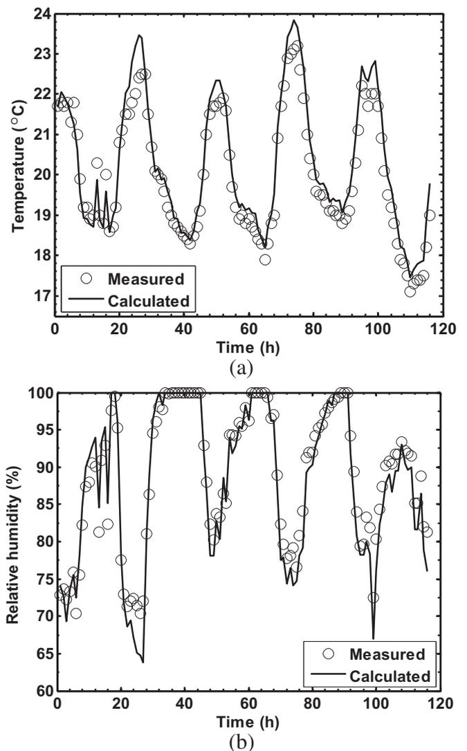
Fig. 6. Comparison of air properties at  $z = 260$  m ( $z/L = 0.84$ ) cross section (a) average cross-section temperature (b) average cross-section relative humidity.
