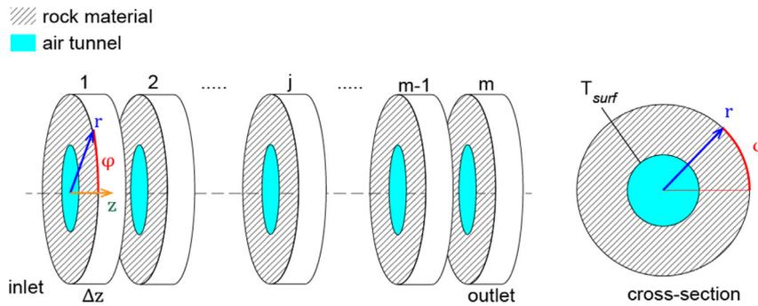
**Fig. 2.** Radial cross-sections of the earth soil surrounding the air-tunnel using cylindrical coordinates. Each cross-section is labeled from 1 to  $m$ , and has thickness  $\Delta z$ , where  $\Delta z \ll r$ .  $T_{surf}$  is the temperature at the surface of the tunnel.
